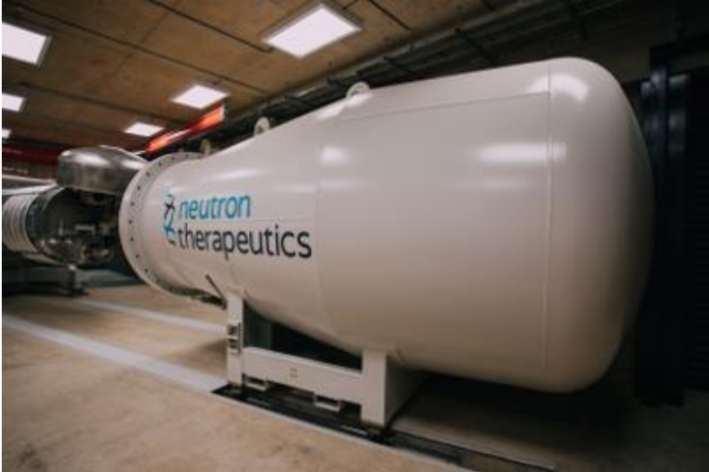
High flux accelerator neutron source for BNCT
